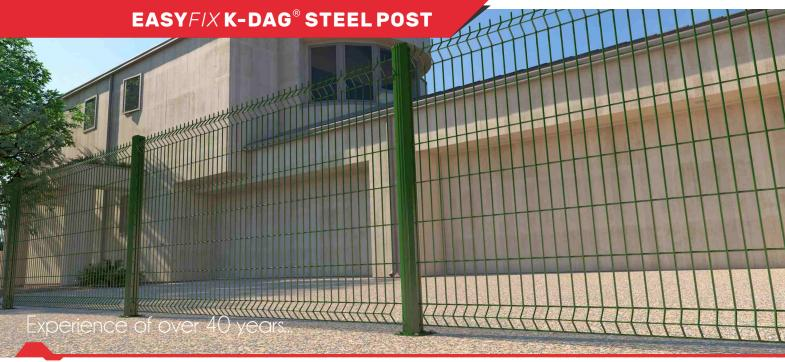
Easyfix K-DAG Steel Post (90x90mm) has been designed to perform maximum strenght with mimimum material to keep it economically. The panels are fixed to post without accessories such as screws, bolts, clips or clamps. As a result it avoids damage on materials during fastening. Slots are at every 100mm and each post is covered with a plastic cap.
